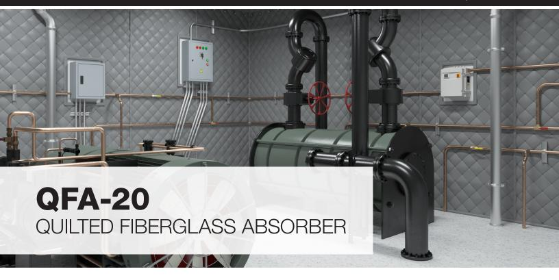
Quilted Fiberglass Sound Absorbers reduce the reflection of sound waves by adding soft, porous, open-celled materials to any environment. The **QFA-20** offers maximum sound absorption performance across all octave band frequencies and is especially effective for rumbling low frequency applications. A vinyl coated fiberglass cloth facing is quilted on both sides of a 4" thick fiberglass core. Wall panels and overhead baffles are constructed with all edges bound and grommets across the top.
